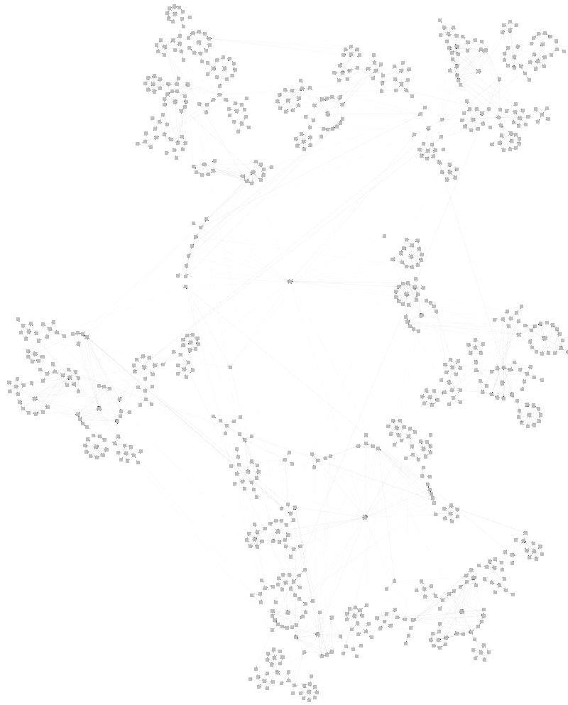
Fig. 6. A backbone balloon drawing of the same Amazon recommendation network as in Fig. 5 with 851 vertices and 4,110 edges.
